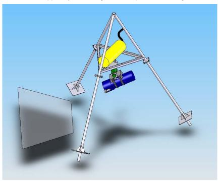
The area shown beside the tripod is the field of view of the camera when it is tilted at 25 degrees and the lens is set at maximum wide angle.
